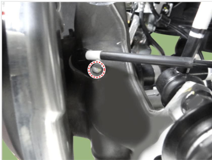
3. Loosen the rear wheel speed sensor bracket bolt.
