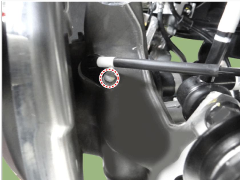
3. Disconnect the ECS connector (A).
