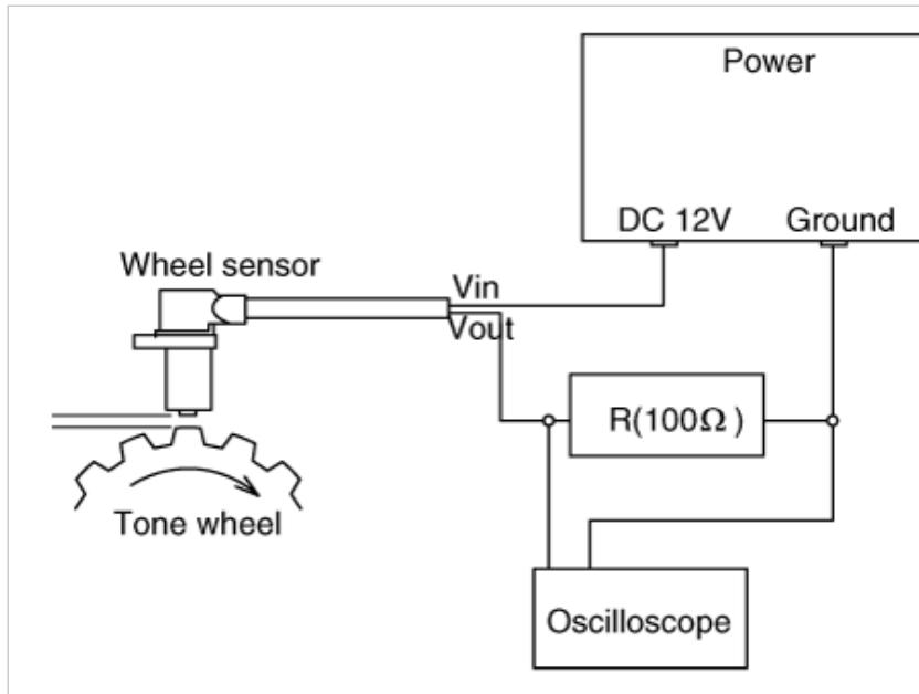
2. Compare the change of the output voltage of the wheel speed sensor to the normal change of the output voltage as shown below.
