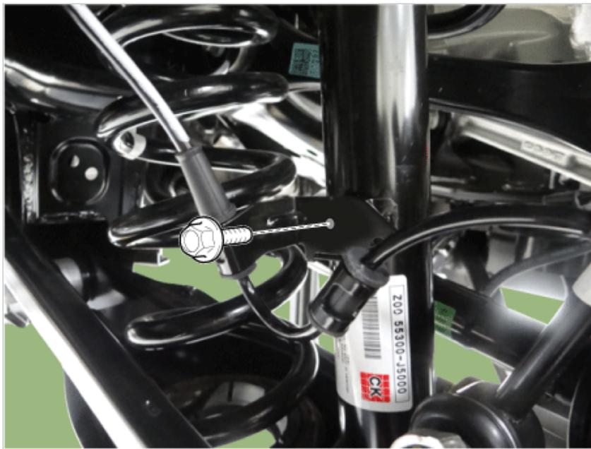
4. Disconnect the rear wheel speed sensor connector.
