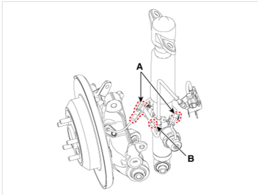
5. Disconnect the rear wheel speed sensor connector.
